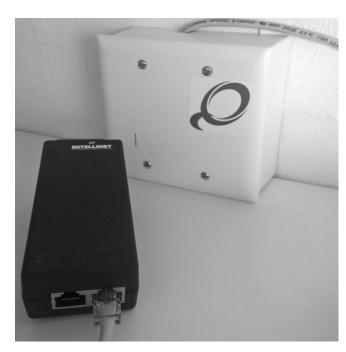
The Team Receiver must be connected via a PoE-Adapter (Power over Ethernet) on the same Ethernet-based Local Area Network as the computer running IQNITER Studio software is connected (i.e., connected to the same Router). A Power over Ethernet connector provides power and Ethernet connectivity using one standard network cable.
