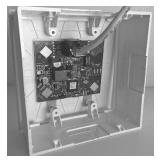
5. Connect the Ethernet cable to the receiver.
